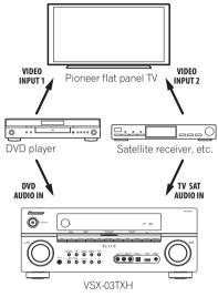
To make the most of the SR+ features, you should connect your source components (DVD player, etc.) in a slightly different way to that described in this chapter. For each component, connect the video output directly to the flat panel TV, and just connect the audio (analog and/or digital) to this receiver.
